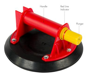
**Before** using the Lifter, ensure that the surface of the material being lifted is free of dirt, oils, grease, water, powders, or other substances, as these will greatly impair the necessary seal created by the Suction Cup Lifter. Also ensure that the face of the rubber suction cup is clean and free of any debris.
